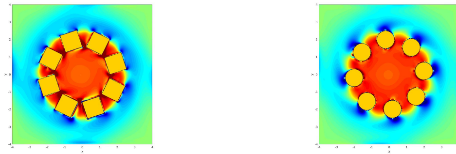
Figure 6.36: Geometry of flow around multiple cylinders rotating around a center
